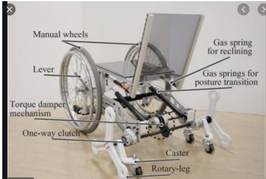
Figure 3.2.1.3 A wheelchair with lever propulsion control for climbing up and down stairs This model provides the full description of the mechanism of the wheelchair. It could inspire the team to explore more prototypes of the subsystem of wheelchairs.
